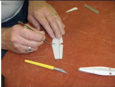
22. Likewise, glue the rudder horn to the rudder. Note orientation.
