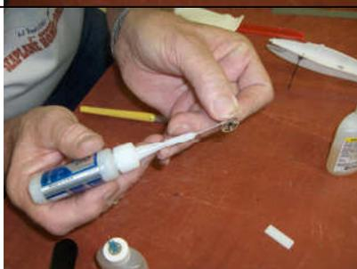
32. After carefully aligning the axels, secure the axel/landing gear/heat shrink with CA.
