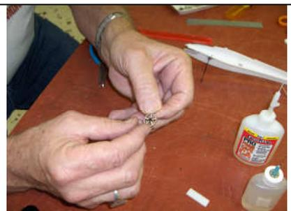
31. Use CA to secure the hubs to the wheels. Be careful to keep CA out of the axle hole.
