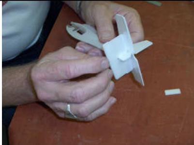
24. After the elevator/stab is aligned, glue with CA and Kicker.
