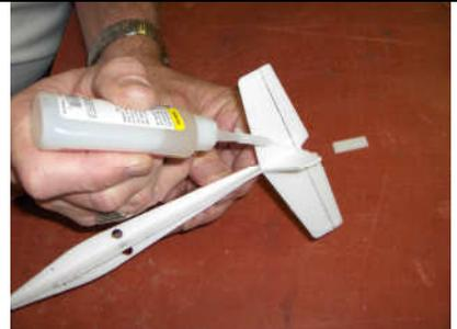
25. Using 3 tape hinges, mount the rudder to the fin/fuselage.
