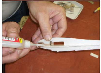
27. Insert and glue the other gear leg. Gear leg should be flush with top of the stiffener.
