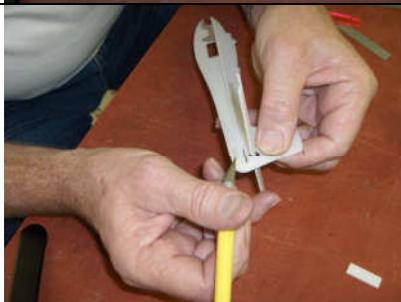
26. Glue one of the gear legs into fuselage. Gear leg should be flush with top of the stiffener.
